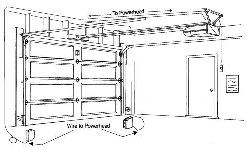
Note: If wires must be lengthened or spliced into prewired installation, use wire nuts or a suitable connector.
